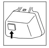
The light sensor is located on the inside of the vehicle at the back of the rearview mirror.
